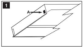
Install 1 small pad (**A**), included in the hardware package, to each side of the main liner plate. (See figures 1 and 2)
